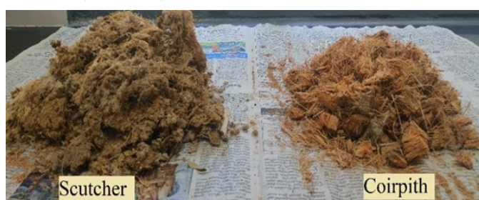
Scutcher, a byproduct of banana fibre extraction process
