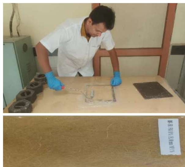
Fig. 36. Nanocellulose-induced banana fibre epoxy composites
